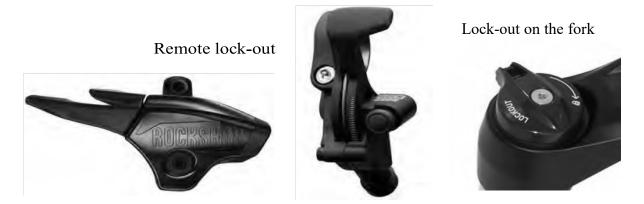
**WARNING!** Do not ride your e-bike with the fork locked-out while off-road, you may lose control and fall, which can cause damage to the fork, serious injury or death! Also note that the fork is not designed for riding in extremely challenging terrain, jumps, downhill, freeride or dirt jumps. Failure to respect this information may result in fork damage, serious injury or death. Failure to respect this information results in loss of warranty.
