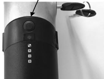
In order to dismount the battery from the frame, turn its key clockwise and pull it out.
